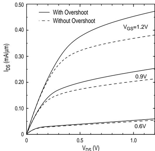
Fig. 3. UFPDB-predicted current-voltage characteristics of the  $L_{eff}=70nm$  bulk-Si nMOSFET with and without velocity overshoot.
