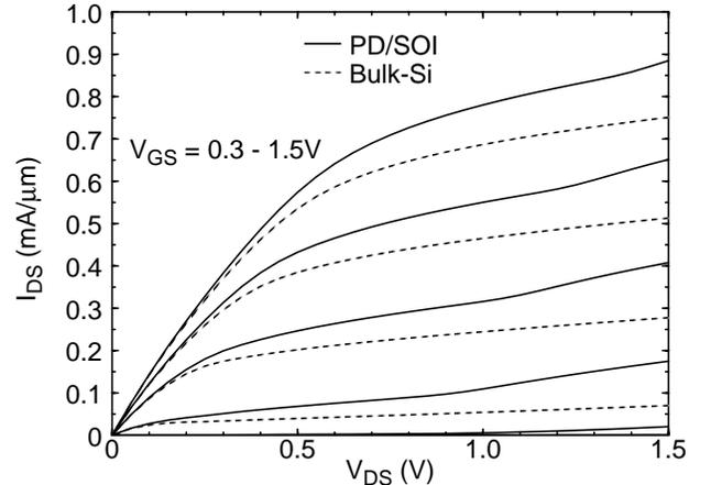
Fig. 2. UFPDB-predicted current-voltage characteristics of  $L_{eff}=70$ nm FB PD/SOI and bulk-Si nMOSFETs.
